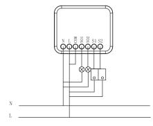
L: Line voltage input N: Line neutral NO1: Switched load1 output NO2: Switched load2 output S1: Connect to wall switch1 input S2: Connect to wall switch2 input COM: Load supply power Input
